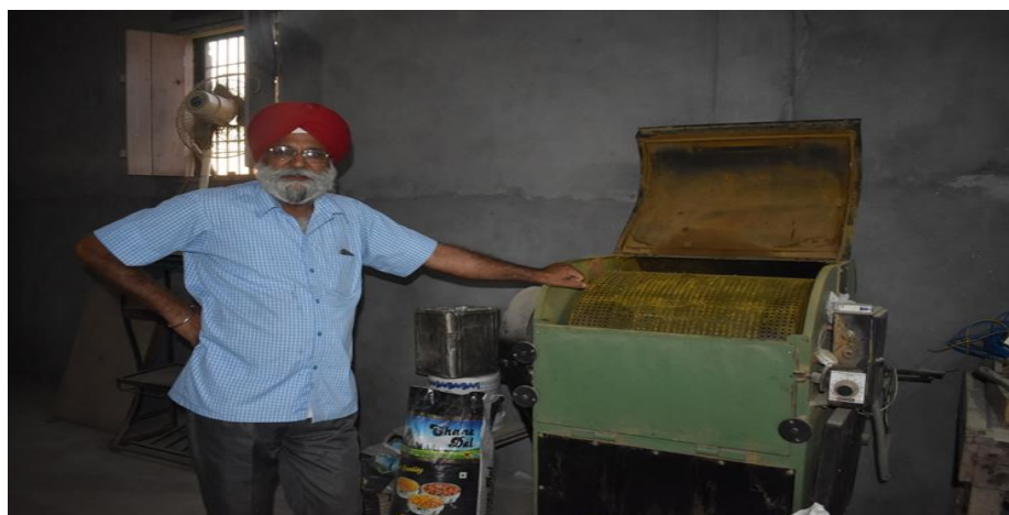
Fig. 5.60: Interior view of polishing machine for turmeric.
