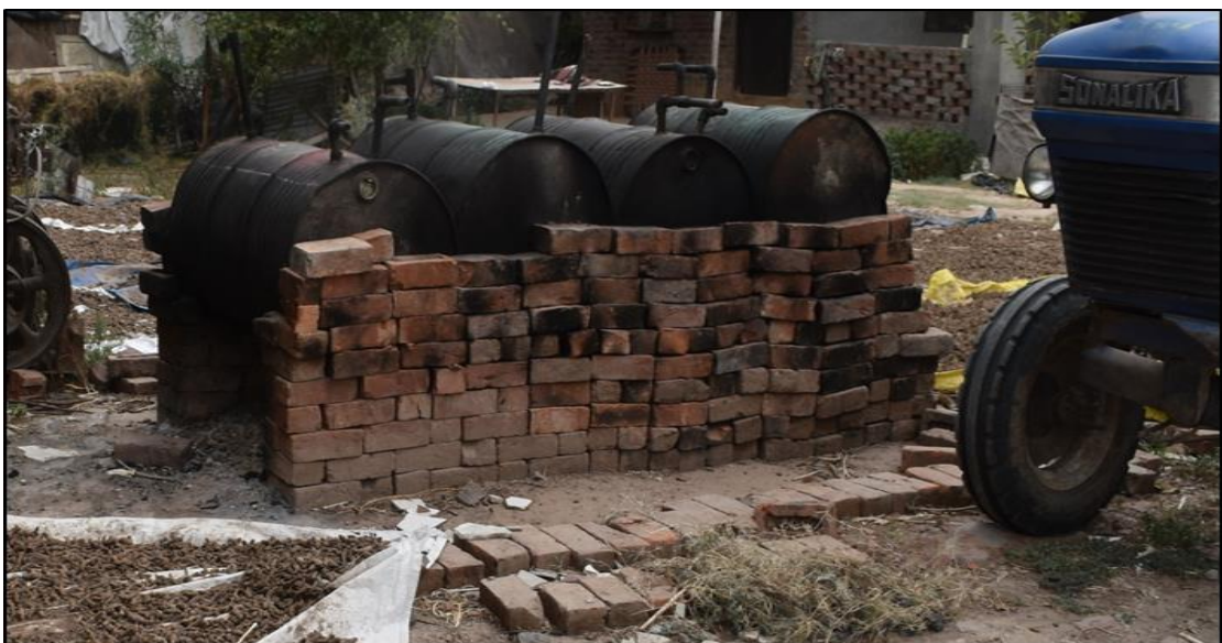
Figure 5.55: Boiling assembly devised by a farmer using drums and connecting vessels.
