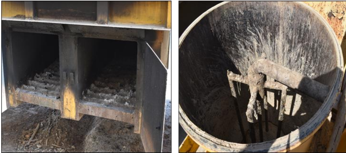
Figure 5.56: Furnace and inner view of vessel of improved turmeric boiler.
